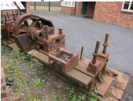
Roll cutting lathe from Wortley Forges
